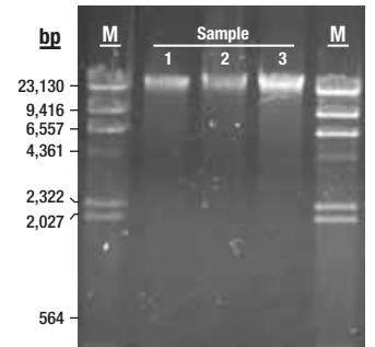
**Figure 1. DNA from 3ml aliquots of HG-BCD sample was purified using the ReliaPrep™ Large Volume HT gDNA Isolation System.** DNA (200ng) was loaded onto a 1% agarose gel and separated at 100V for 40 minutes. M = Lambda DNA/HindIII Markers (Cat.# G1711).
