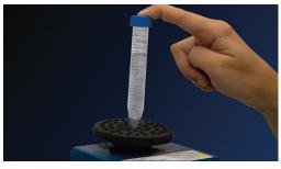
**Figure 6**: Vortexing the sample for 30 seconds will allow you to recover DNA smeared on the side of the tube. The DNA will remain high molecular weight.
