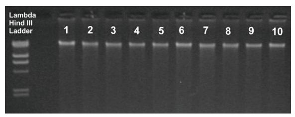
Figure 7: Representative agarose gel showing high molecular DNA.
