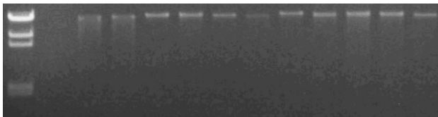
Figure 2: Agarose gel electrophoresis (0.8% agarose, 90 V, 60 min) of DNA from 10 canine samples purified within 72 hours of sample collection. A Lambda-HindIII digest was used as a marker in Lane 1.
