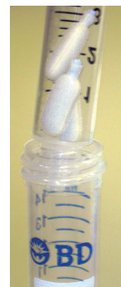
Figure 1: Syringe barrel with sponges inserted in conical tube for centrifuge.
