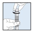
Close tube tightly with small cap. Shake for 5 seconds.
