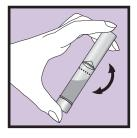
Shake the capped tube for 5 seconds.
