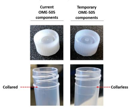
**Reason for change:** The OME-505 is being used to fulfill large volume OMNIgene•ORAL COVID-19 orders. In response to the increased demand for these devices for COVID-19 testing, DNA Genotek is temporarily implementing manufacturing efficiencies to allow for improved product supply to customers.
