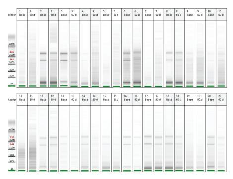
Figure 1. Room temperature post-collection RNA stability. Bioanalyzer images for each of N = 20 samples collected in ORAcollect•RNA devices aged for 13 months at  $27^{\circ}$ C  $\pm 2^{\circ}$ C pre-collection, showing baseline extraction (Base) and 60-day post-collection extraction (60 d) side by side for each collected sample. Ladder fragment sizes are shown as total number of bases. Approximate location of 16S and 23S ribosomal RNA bands is indicated on the ladder in red font.
