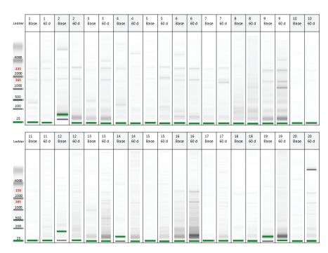
Figure 2. Simulated transport post-collection stability. Bioanalyzer images for each of N = 20 samples, showing baseline extraction (Base) and 60-day post-collection extraction (60 d) side by side for each collected sample. Ladder fragment sizes are shown as total number of bases. Approximate location of 16S and 23S ribosomal RNA bands is indicated on the ladder in red font.
