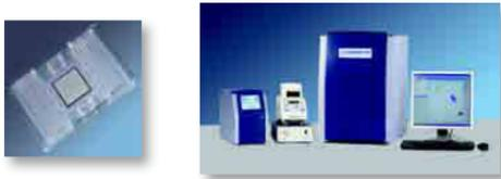
Each 96.96 Dynamic Array IFC (left) is capable of running 96 samples against 96 SNP assays generating a total of 9,216 genotypes. The advantages include:
